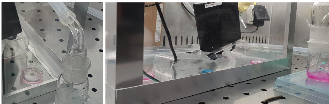
Figure 5 – Positioning of two 35mm cell-culture dishes containing 1 mL of RMPI to evaluate possible viral settling down during nebulization and ionization
